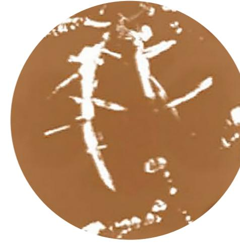
Strongly heterogeneous nucleation at the surface associated with small undercooling
