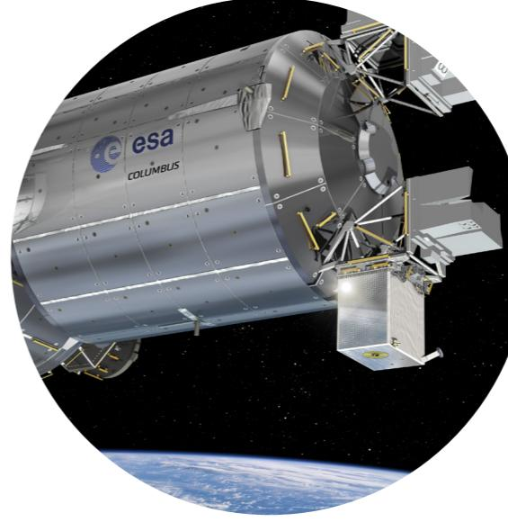
Atomic Clock Ensemble in Space (ACES) facility attached to the Columbus module on the International Space Station.
